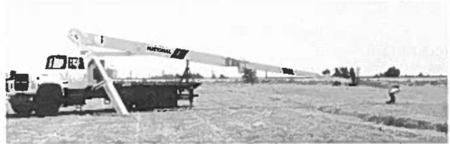
This photo sequence demonstrates how a National jib folds out into working position.
